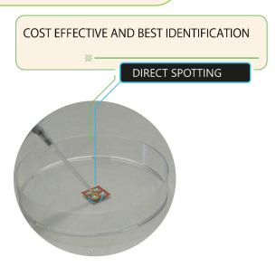
Simply put a  $10\mu L$  drop of your sample suspension either from a colony from your plate or isolated from your unfilterable matrix onto the sample substrate. On a  $40^{\circ}C$  plate it dries up in just 5 min. Makes this the perfect sample for immediate isolate ID or database updates.
