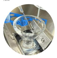
With volume from 0,1 to 500 mL you can prepare a sample for analysis with a flowrate of 4-16 mL/minute. mibiC's reusable easy to use and easy to clean & autoclave filtration system ensures the highest recovery rates.
